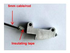
4. Slide the hook to the masttop, paying attention that it does not twist around its axis, but keeps its "nose" towards the leading/foreward egde of the mast.
